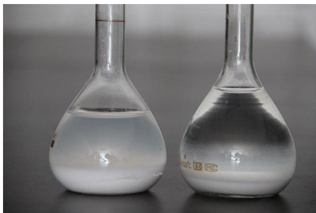
Fig. 2. Photographs of cationic starch modified filler slurry (left) and cationic starch/carboxymethyl cellulose modified filler slurry (right) after storing at room temperature for 24 h
