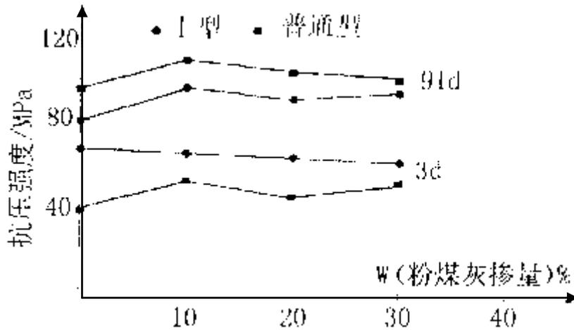
Figure 3.3 Effect of Fly Ash on the Compressive Strength of Mortar
