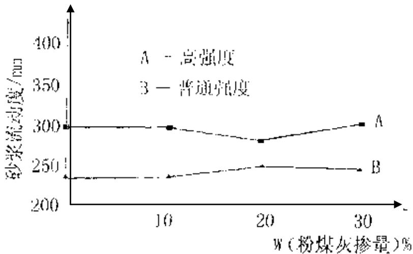
Figure 3.2 Effects of Fly Ash on the Fluidity of Ordinary Portland Cement Mortar
